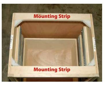
2. You mount the top to the base units by screwing directly up through the wooden mounting strips from below.
