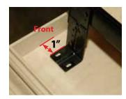
3. The front edge of the keyboard bracket should be 1" back from the rear edge of the front desktop trim. Center the keyboard slide from side to side . Note: The keyboard slide can be positioned where you desire, left or right.
