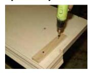
In some instances, there is not enough clearance space between the bottom of the desk trim moulding and the keyboard slide, causing your keyboard to hit on the desk trim. In these cases, addition spacer blocks can be installed to create more space between the keyboard slide and the desktop. Simply attach the spacer blocks using two 1 1/4" course wood screws.
