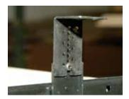
2. The legs of the keyboard slide are adjustable; simply remove the screws, and adjust to the desired height. Reattach screws.
